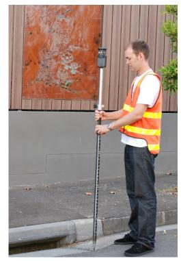
Authorities and councils are currently utilising GPS technology to capture their existing assets. GPS technology may provide unreliable data sets due to the accuracy limitations of the technology. Beveridge Williams can provide a quality audit of these processes and an error analysis to ensure the required accuracy of the data is being achieved.
